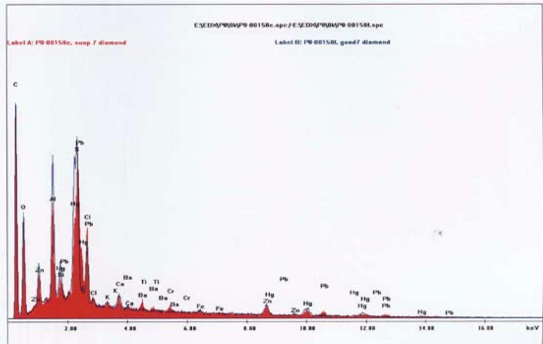
**Figure 9.** The elements found in the left and right “7” numbers of a “77” pair on the cover.
